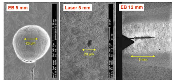
Fig.6: Typical drawbacks of beam welds (especially EB) are pores. In thicker plates even large unbonded areas have been observed (right image).
