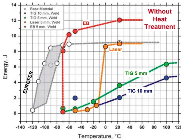
Fig.3: Charpy properties of the different welds without post welding heat treatment. The EB weld is nearly as good as the base material.
