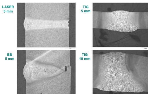
Fig.1: Microstructure of the different welds. It can be seen that the intensity of the EB was too low to for a complete fusion of the beam stopper. Therefore, the V-notch has been placed on this side for fabrication of Charpy specimens.
