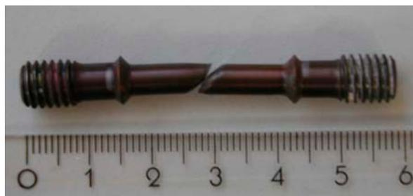
Fig.5: Creep properties of TIG welds suffer from distinct gliding along softened HAZ. In this example test parameters have been 600 °C, 140 MPa and time to rupture has been 74 h (for comparison, rupture time of the base material is 512 h).
