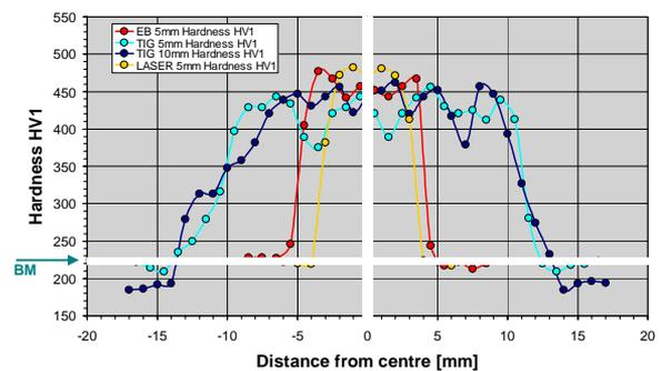
Fig.2: Hardness profile of the different welds. Typical for TIG welds are the softened regions around the HAZ and the broad lateral extensions. The hardness level of the base material is marked with an arrow (BM).
