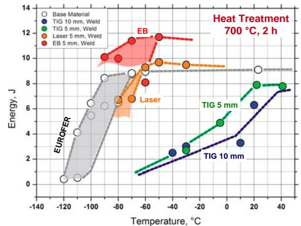
Fig.4: Charpy properties of the different welds after post welding heat treatment of 700°C/2h. DBTT of Laser and EB welds are nearly comparable to the base material.
