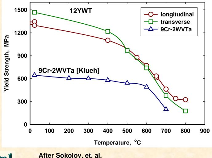
Mechanicalalloying (MA) of fine prealloyed metal and Y<sub>2</sub>O<sub>3</sub> powders used to produce very high strength oxidedispersionstrengthened alloy of 12Cr-3W-0.4Ti +  $0.25Y_2O_3$
