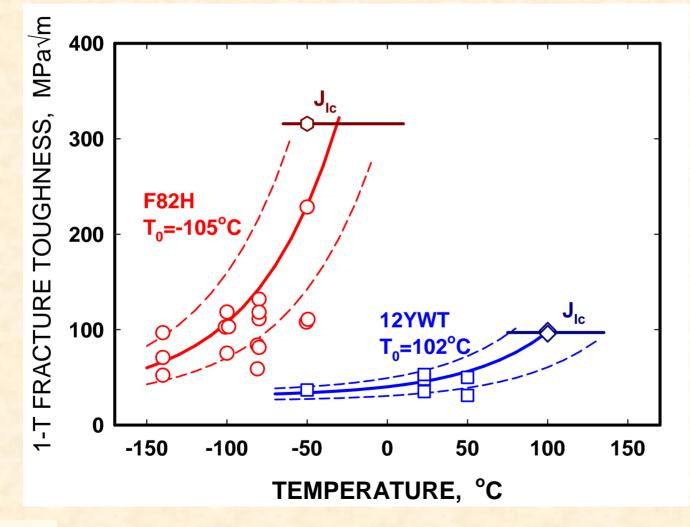
Three-point bend specimens 1.6×3.2×25 mm were used for fracture toughness testing of 12YWT
