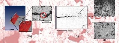
XMT enables crack propagation mechanisms to be studied in situ. The figures show that both crack bridging (m) and microcracking (n) toughening mechanisms are in operation. A stable bridging zone behind and process zone ahead of the crack tip enable the form of the R-curve to be understood. The effect of graphite microstructure (filler size and shape, porosity) on properties can be found.
