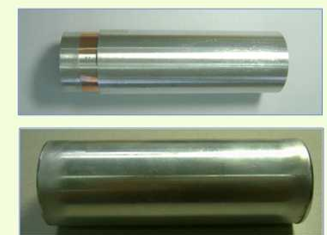
Proto-type ^{99}\text{Mo} target, fabricated by welding of Al tubes
