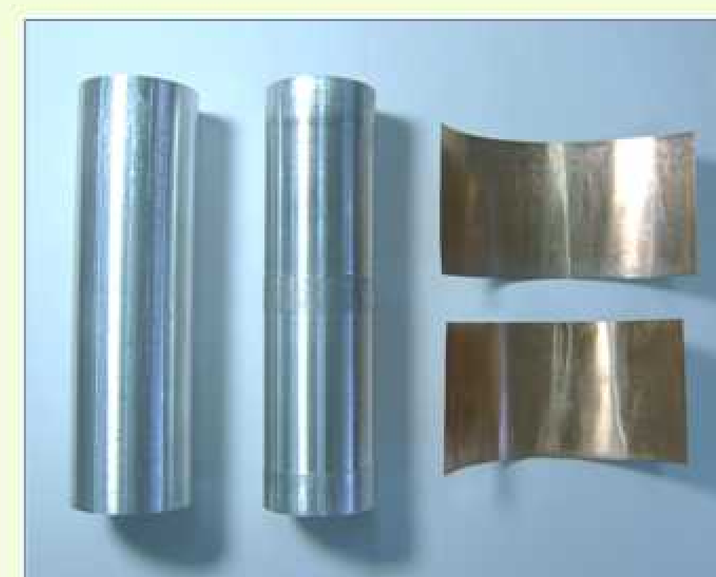
Proto-type ^{99}\text{Mo} target, fabricated by welding of Al tubes
