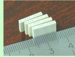
Nanoceramic cases of microwave duplexers from (\text{Ba,W})\text{TiO}_3
