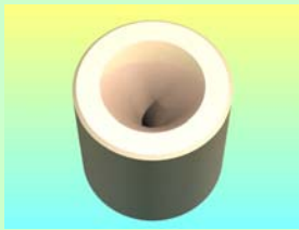
Die for first drawing from Y-TZP nanoceramics
