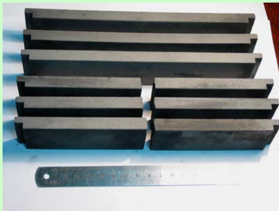
Die for first drawing from Y-TZP nanoceramics
