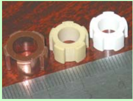
Impellers for the gasoline pump from Y-TZP nanoceramics
