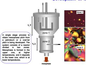
After 6 h of reaction, in the upper part of the reactor (zone 1), very little mesophase is observed. In the middle part, the mesophase content increases significantly. The diameter of the spheres is much larger than in zone 1.The lower part (zone 2) contains a highly pure mesophase pitch, fully coalesced, proving the viability of the method. Moreover, the process has the potential to extract the mesophase continuously from the reactor.
