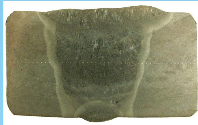
Figure 1. Macrostructure of C weld joint after PWHT
